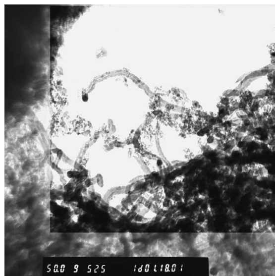
Fig. 9. TEM image (50,000 \times ) of 12 wt.% Co/SiO 2 after reaction in 5% CH 4 /0.4% CO/Ar at 773 K for 60 min showing presence of filamentous carbon with diameter \sim 25 nm.
